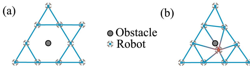
Figure 5.4: A demonstration of how more edges can degenerate collision avoidance. (a) shows a configuration with 14 edges, whereas (b) shows the same configuration with 18 edges. The red robot is pulled towards the centre of its neighbourhood, but this degenerates its ability to avoid the obstacle in the centre of the flock. Image from Zhang et al. (2025).
